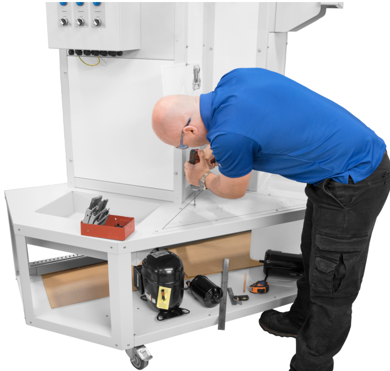
Figure 24. Technician drilling the mounting holes in the horizontal plate.
