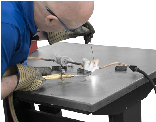
Figure 19. View of the brazing technique.
