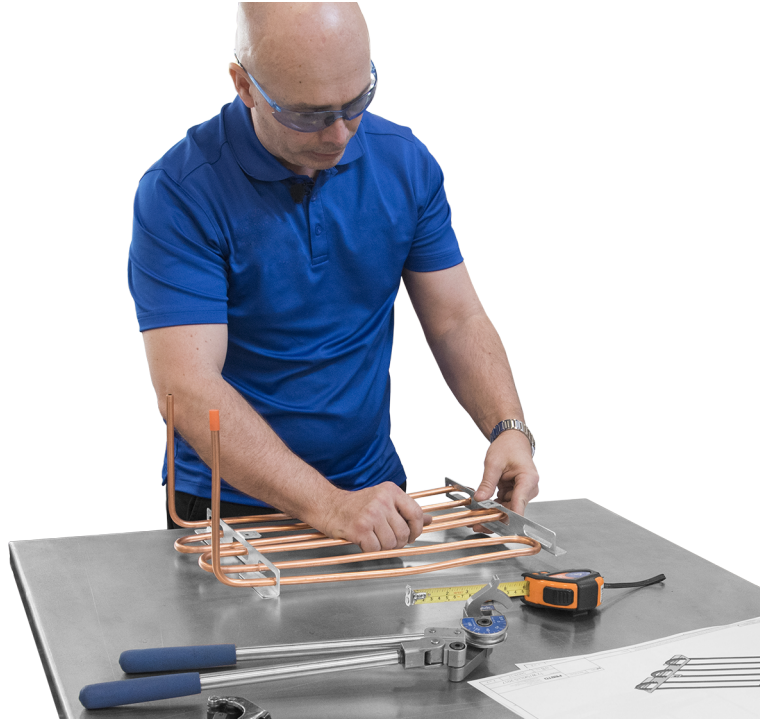
Figure 11. Technician assembling the evaporator coil.
