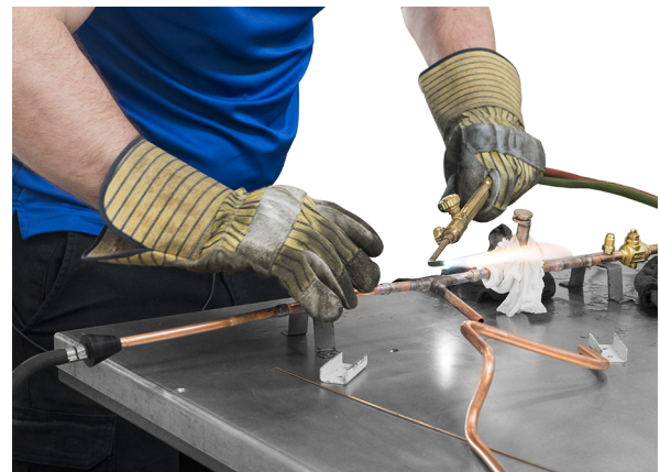
Figure 20. Technician brazing the heat recovery circuit.
