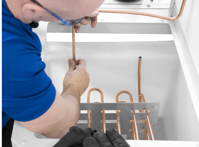
Figure 21. Technician inserting a branch of the heat recovery circuit in a piping of the heat recovery coil.
